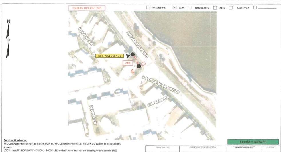
LOC 4: Install 1 ROADWAY - 7,500L - 3000K LED with 6ft Arm Bracket on existing Wood pole in (NE orientation.
