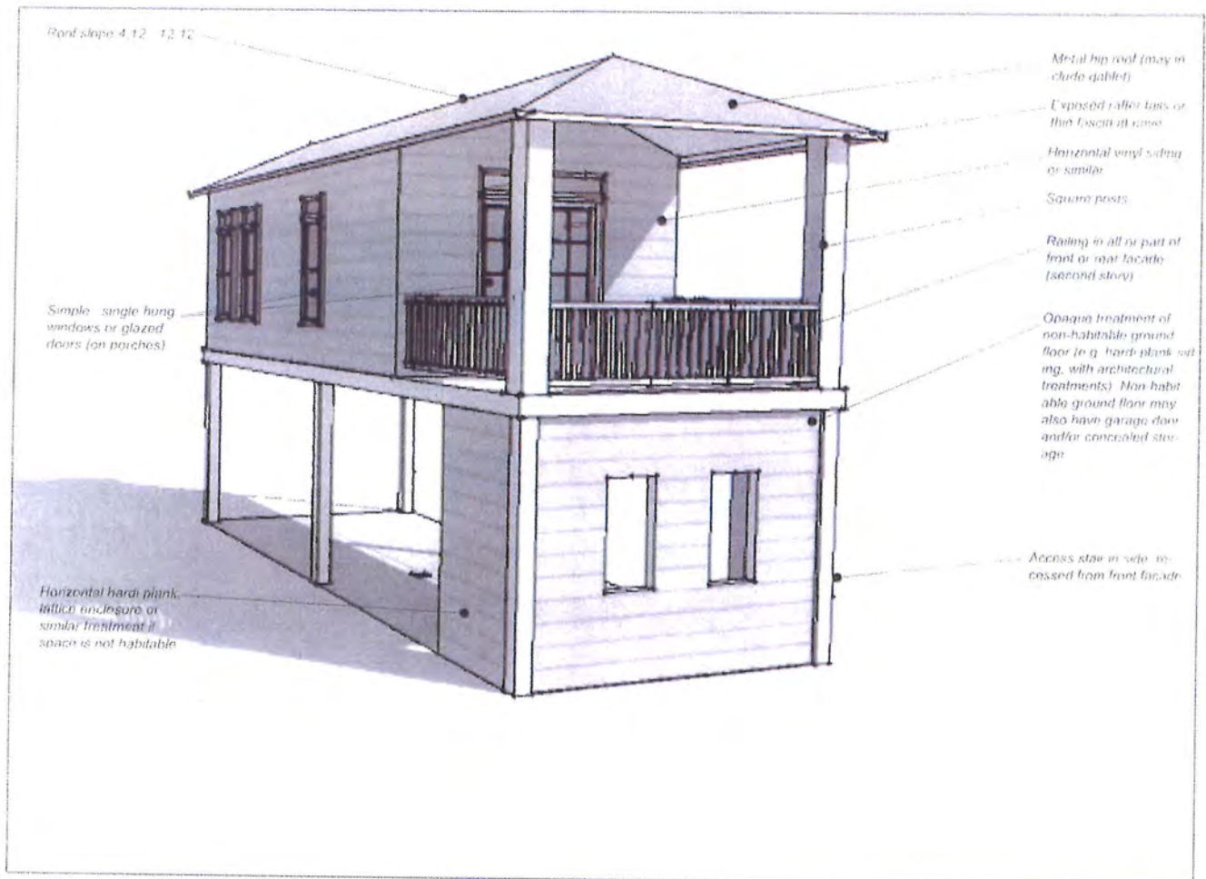
Figure 17.3 Building Elements - Elevated Single Story
